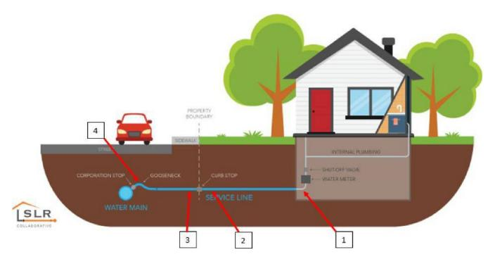
Each service line requiring verification **must have the following three or four points physically verified** (numeric bullets refer to the numbered location in the illustration above):
